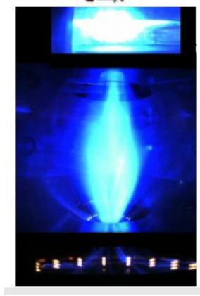
FIGURE 1. Image of PROTO-SPHERA plasma in Argon as reconstructed from three cameras: anodic region (top), the nearly cylindrical region (middle) and cathode (bottom). View at transitions from linear to mushroom-shaped regions is impeded by coils. The mushroom-shaped plasma is clearly visible in the anodic region at the top. The cathode region luminosity is dominated by hot electron emitters (visible as brilliant spots).
